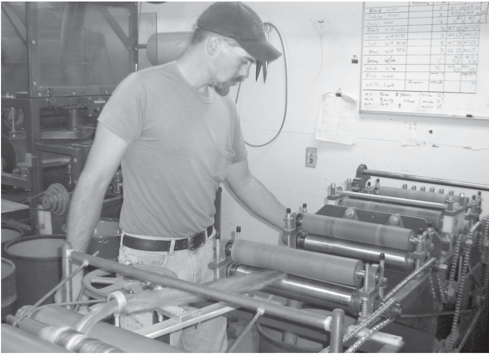
Jeremiah Squier keeps an eye on the draw frame at Twist of Fate Spinnery.
